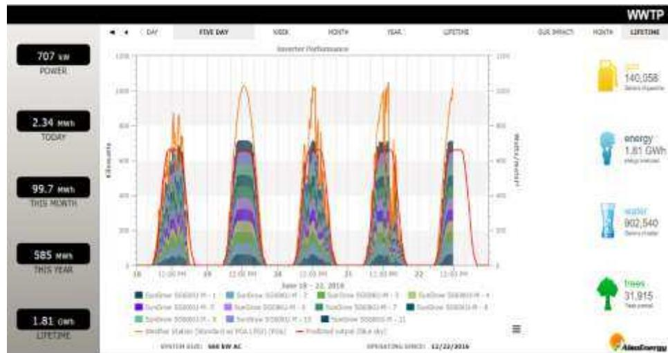
To provide additional insurance against downtime and underperformance, each inverter and segmented portions of the system (zones) report independently of the overall meter monitored production. The system is then configured with production alerts that are triggered in the event of a system failure or
