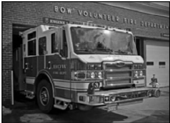
Because of height constraints in the garage door opening, contemporary equipment must be custom built for the Bow Fire Department at an added cost. (Photo by Eric Anderson)
